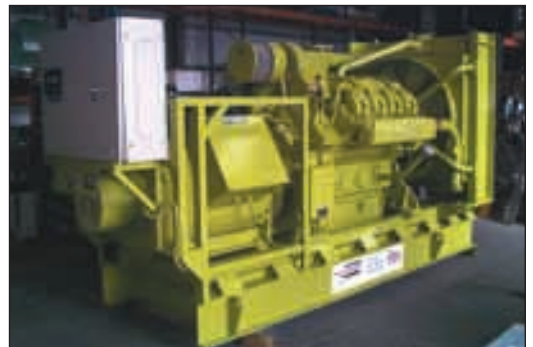
A completed 500kVA Rolls Royce
