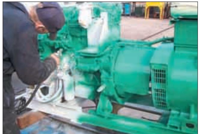
A generator undergoing spray painting
